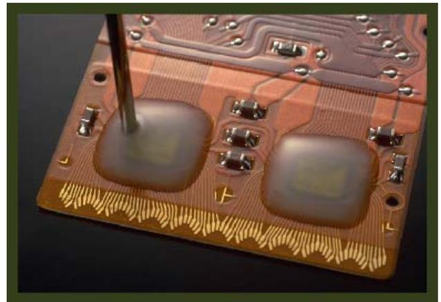
Photo: **UVE-1017-2** on a polyimide flexible circuit.
